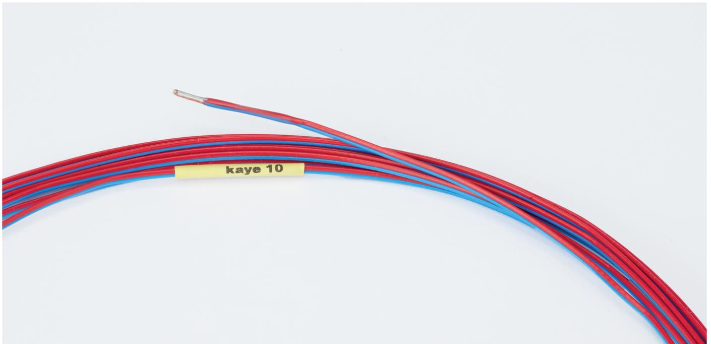
The Ultra-Premium Grade Autobond Thermocouple Wire was designed to eliminate leakage of water or steam through standard Teflon thermocouples. The Autobond wire eliminates the outer clear Teflon jacket which is where 90% of moisture creep occurs and also creates a mold on the inner wires which eliminates any inner air pockets for moisture to flow.
